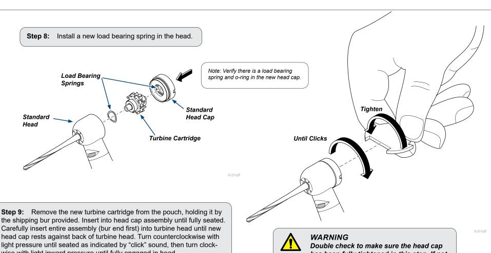
wise with light inward pressure until fully engaged in head.
